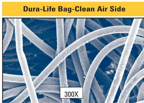
These photos were taken with a scanning electron microscope of bag media used in a collector that was filtering fly ash. The bags were removed after 2,700 hours of use. Air-to-media ratio was 4.5 to 1. Pressure drop was 6 in. on polyester bags and 2 in. on Dura-Life.
